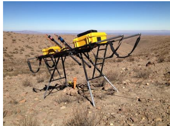
Figure 3: Example of ADR field equipment ready for conducting a Stare scan in a rugged terrain with the antennas positioned at an angle.
