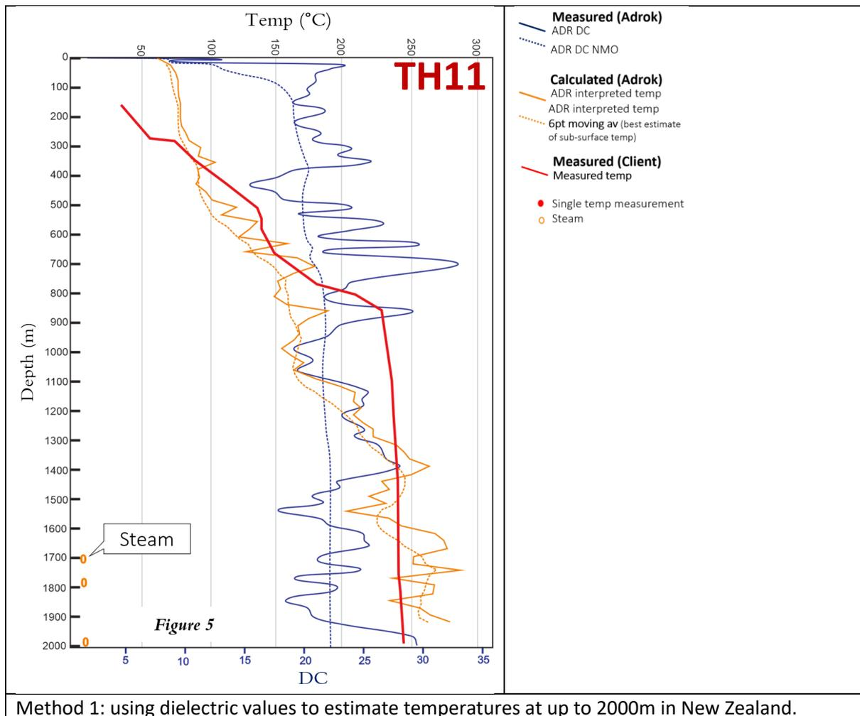
Method 1: using dielectric values to estimate temperatures at up to 2000m in New Zealand.
