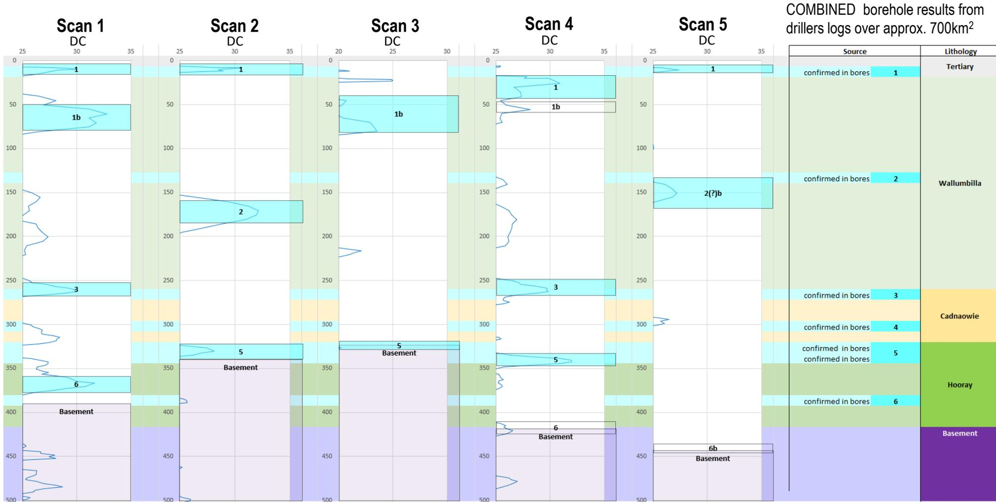
Blue line on all charts shows DC measurements with increasing depth
