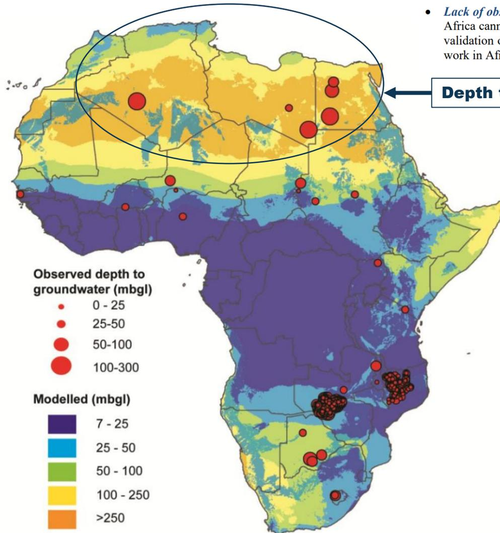
**Depth to groundwater model based on only 6 points**
