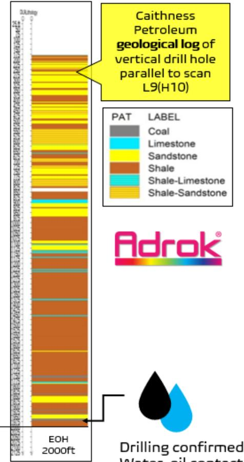
Very high values for correlation in 5-10MHz bandwidth (1 maximum at 1953.45ft) support the presence of oil between 1940-1950ft deep. Combined with other ADR results and when used together, the multiple datasets support the presence of oil and water near the anomaly at 1968ft depth. Drill hole data confirmed water-oil contact at approximately 1955ft depth.
