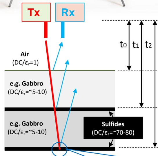
Transmitted pulse (red) is reflected from boundary (blue) between sulfides and host rocks. The strongest reflections occur at boundaries between rocks with greatest contrasting Dielectric Permittivities ( $\epsilon_r$ ) or Dielectric Constants (DC).
