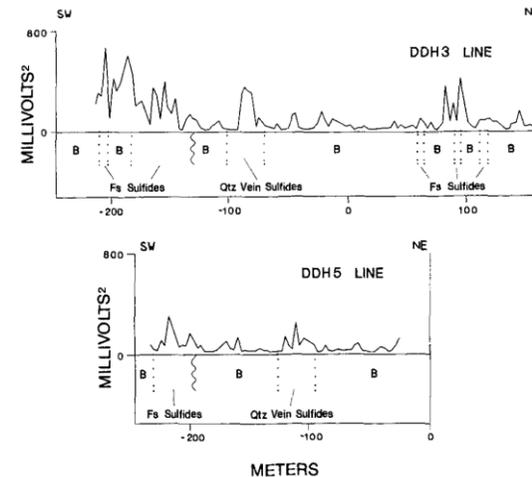
FIG. 4. Radar bottom echo strength and drill hole results on the Mt. Henry Clay Glacier. The echo strength plotted is the squared peak-to-peak amplitude. See Figure 2 for line locations and a plan view of subglacial geology. B = basalt and andesite; Fs = felsic schist.
