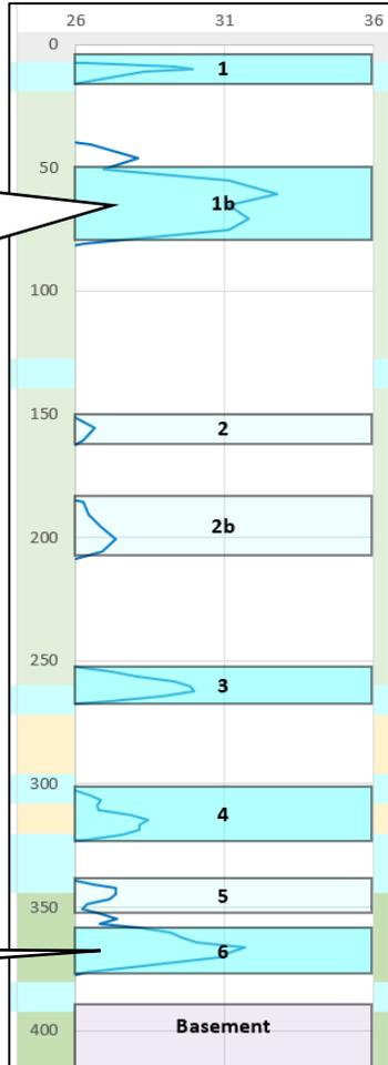
~20m of "Clay Sticky Waddy" recorded in drill logs. Saturated clay with high DC. Also potential aquifer (not logged by driller)
