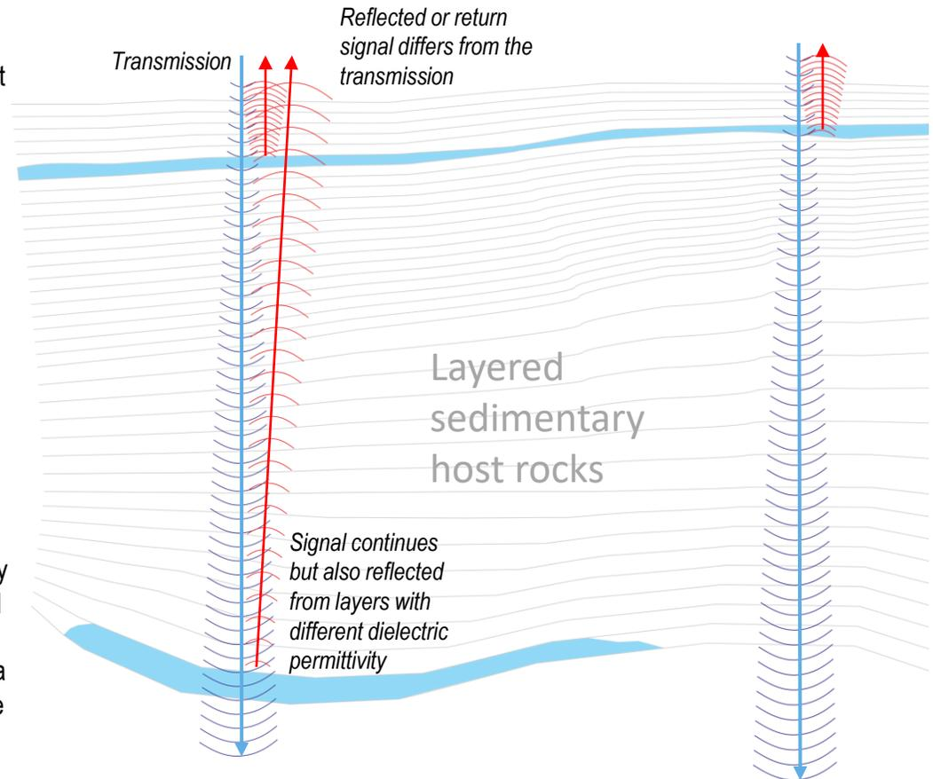
The following experiment was carried out in collaboration with Teck Resources as a test of Adrok's technology to be able to penetrate significant thicknesses of rock and detect materials with different Dielectric Permittivities.
