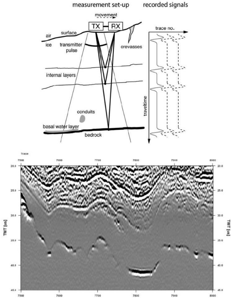
Fig. 11.6. Example of radargram showing a subglacial lake, corresponding to the bright nearly flat reflector in the lower part of the figure around trace 7800, also showing a very low reflection at the steep flanks of the lake. Image courtesy of Daniel Steinhage, AWI.
