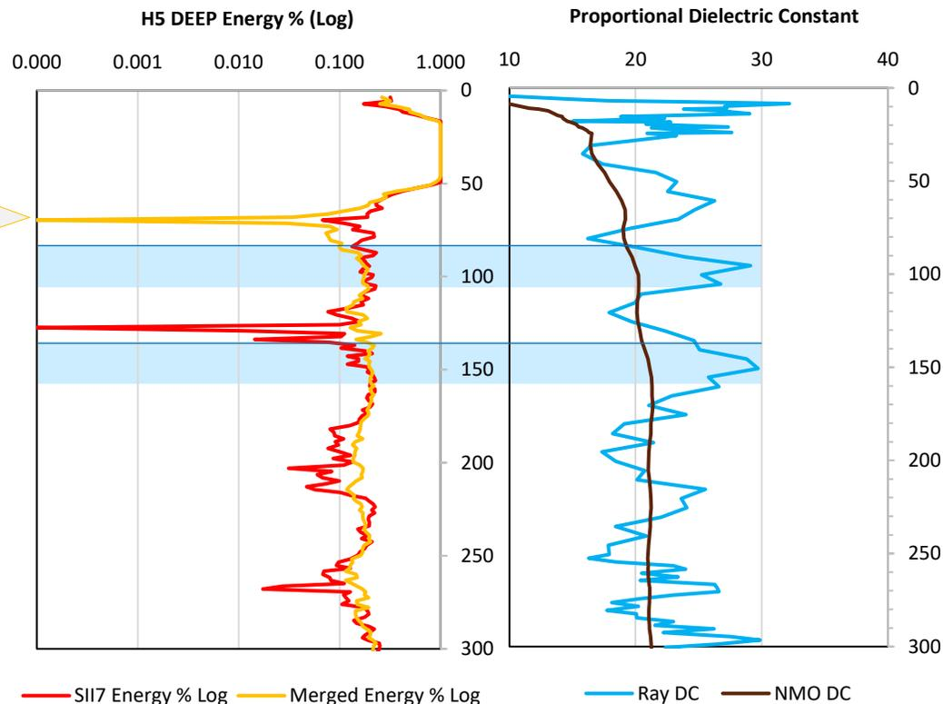
A real-world case example from an Adrok survey where water-saturated sediments are interpreted at around 100 and 150m depth.
