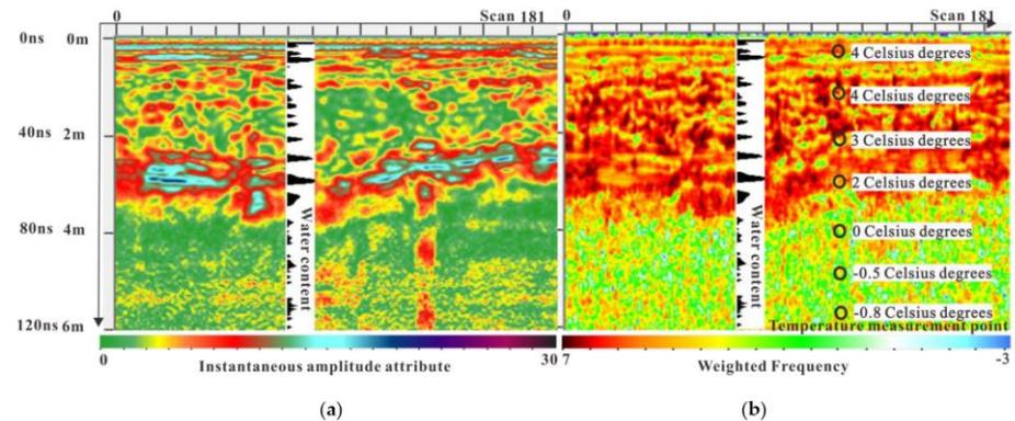
**Figure 9.** Correspondence diagram between electromagnetic wave attribute and measured data. (a) Absolute instantaneous amplitude attribute; (b) weighted average frequency attribute; water content is inserted in (a) and (b); black circle notes temperature in (b). The dielectric constant of the medium is 11.
