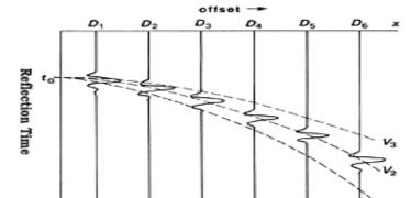
Transmitter & Receiver Normal Move Out (NMO) with increased distance
