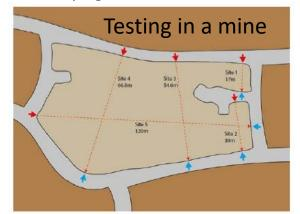
Figure 1: Location of emitters (red) and receivers (blue) for the trans illumination experiments.
