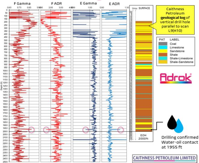
Adrok were contracted to carry out a test of the deep penetrating pulsed radar at detecting oil in Oklahoma for Caithness Petroleum Limited. Results returned a strong anomaly in frequency (F-Gamma and F-ADR) and Energy (E-Gamma and E-ADR) at 1967ft. Ciathness confirmed the water-oil contact at 1955 feet, a difference of 8ft.
