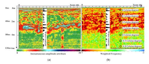
**Figure 9.** Correspondence diagram between electromagnetic wave attribute and measured data. (a) Absolute instantaneous amplitude attribute; (b) weighted average frequency attribute; water content is inserted in (a) and (b); black circle notes temperature in (b). The dielectric constant of the medium is 11.
