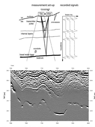
Fig. 11.6. Example of radargram showing a subglacial lake, corresponding to the bright nearly flat reflector in the lower part of the figure around trace 7800, also showing a very low reflection at the steep flanks of the lake. Image courtesy of Daniel Steinhage, AWI.
