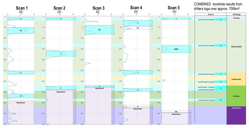
Blue line on all charts shows DC measurements with increasing depth
