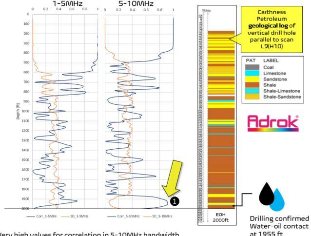
Very high values for correlation in 5-10MHz bandwidth (maximum at 1953.45ft) support the presence of oil between 1940-1950ft deep. Combined with other ADR results and when used together, the multiple datasets support the presence of oil and water near the anomaly at 1968ft depth. Drill hole data confirmed water-oil contact at approximately 1955ft depth.
