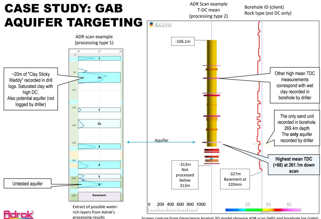
Screen capture from Geoscience Analyst 3D model showing ADR scan (left) and borehole log (right)
