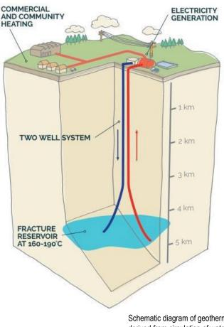
Schematic diagram of geothermal energy derived from circulation of water through hot bodies of rock (typically granites) at depths of up to 5km
