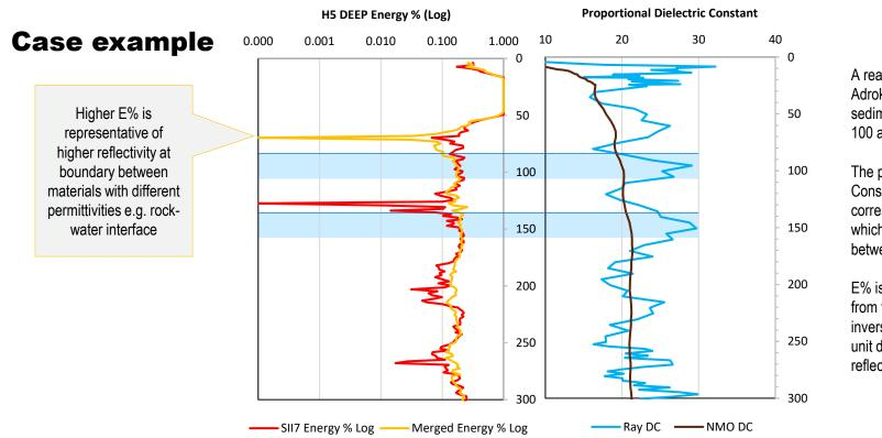
A real-world case example from an Adrok survey where water-saturated sediments are interpreted at around 100 and 150m depth.
