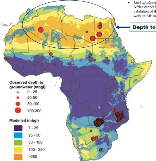
**Figure 6** from - http://nora.nerc.ac.uk/id/eprint/17907/1/OR11067.pdf Comparison of observed and estimated depth to groundwater.
