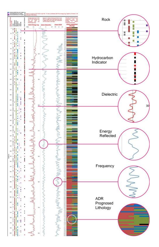
Fig 4. ADR Spectral Lines based on energy v's frequency measurements ("Spectroscopy")
