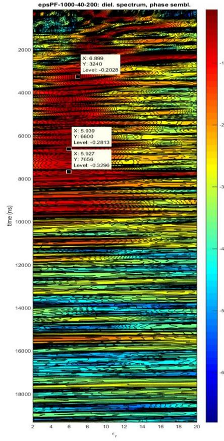
Dielectric can be estimated until about 75000ns at 5.9. Reflection from STARE localized at depth  $3e8/\sqrt{5.9} * 15340e-9/2 = 947m$ .
