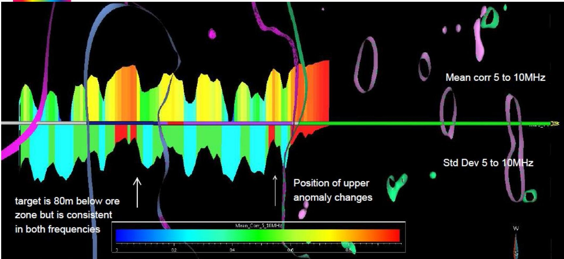
🌟 The two frequency bands for the 1-5MHz and 5-10MHz correlation and standard deviation profiles match up well.
