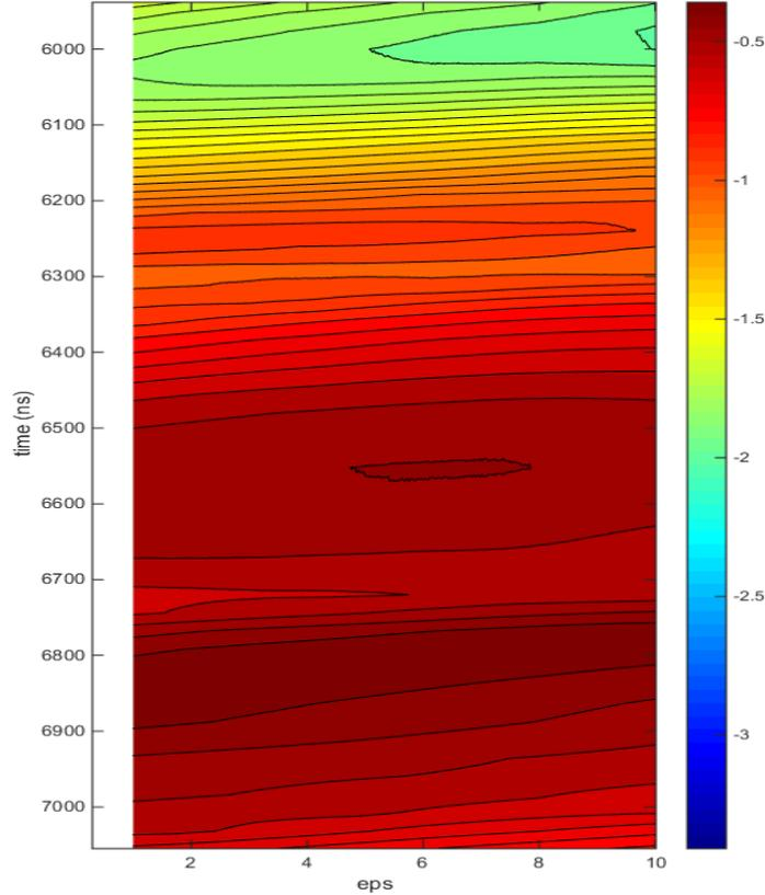
Dielectric constant readings are obtained from visually identifying peaks in the (time, eps) false color plot, which correspond to previously identified reflectors.
