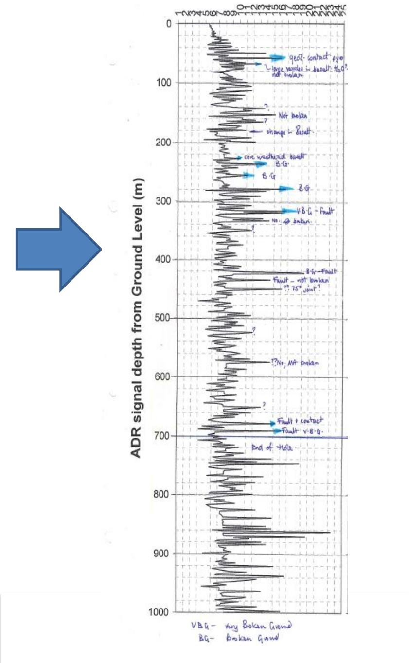
The high dielectrics verified by client from core inspection to be broken ground, very broken ground or faulting (caused by moisture)
