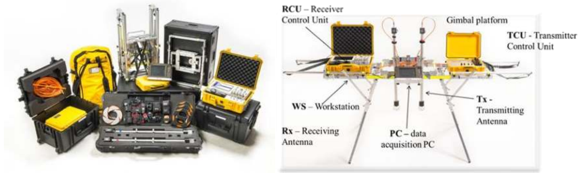
Figure 1: ADR field equipment “ADR Scanner” with rechargeable solar powered portable batteries.
