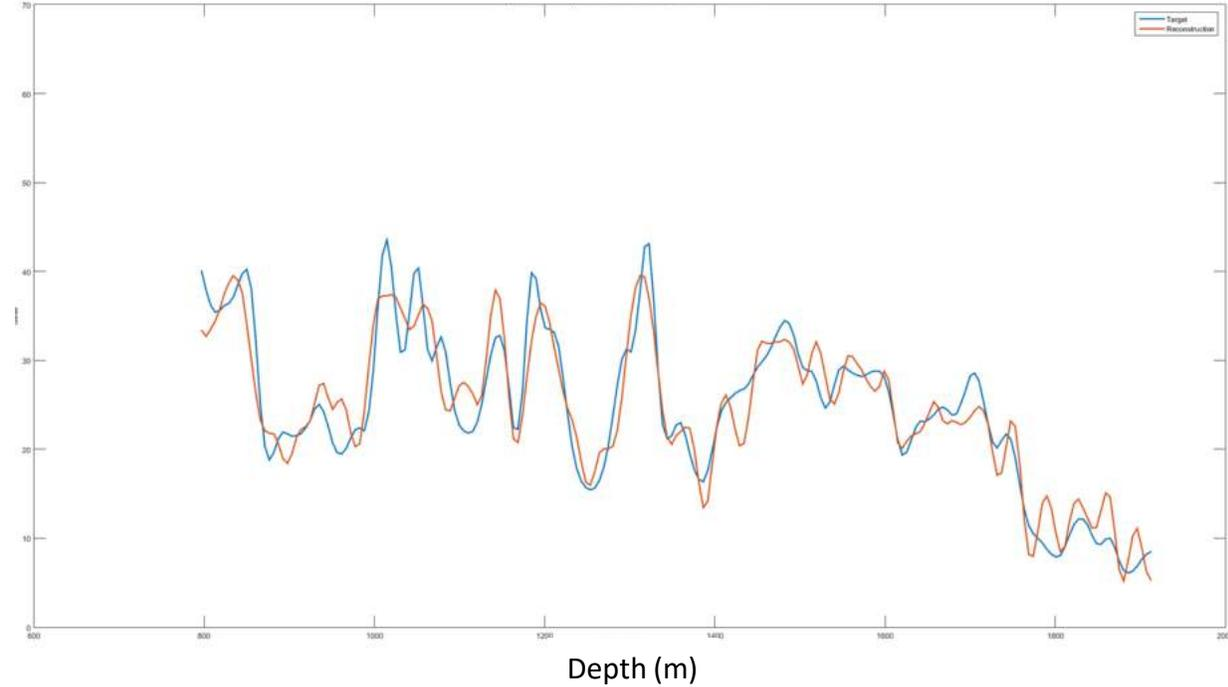
🌈 The CalcData Mix for Neutron Porosity at Ellesmere Port shows a correlation of 81% using a 4 Smooth & correlation of 94% for an 8 Smooth.
