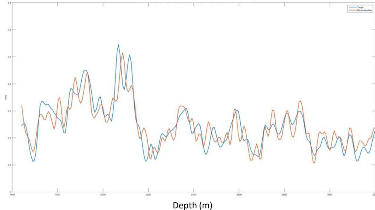
🌈 The CalcData Mix for Neutron Porosity at Becconsall shows a correlation of 66% using a 4 Smooth & correlation of 87% for an 8 Smooth.
