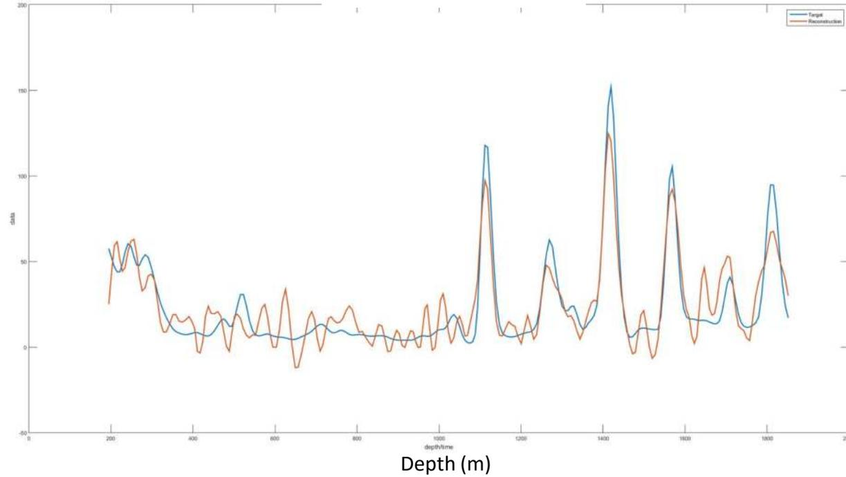
🌈 The CalcData Mix for Deep Resistivity at Bletchingley 1 shows a correlation of 73% using a 4 Smooth & correlation of 90% for an 8 Smooth.
