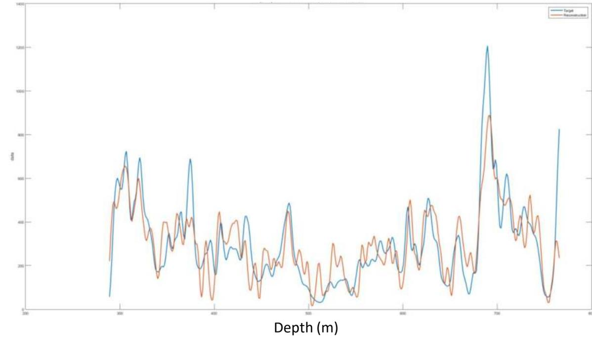
🌈 The CalcData Mix for Formation Resistivity at LF10 shows a correlation of 73% using a 4 Smooth & correlation of 82% for an 8 Smooth.
