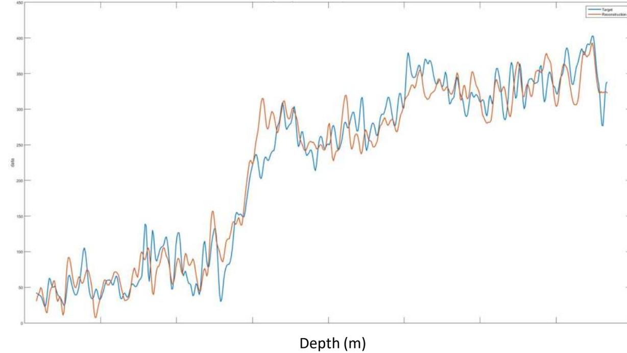
🌈 The CalcData Mix for Gamma Ray at LF03Pt4 shows a correlation of 95% using a 4 Smooth & correlation of 97% for an 8 Smooth.
