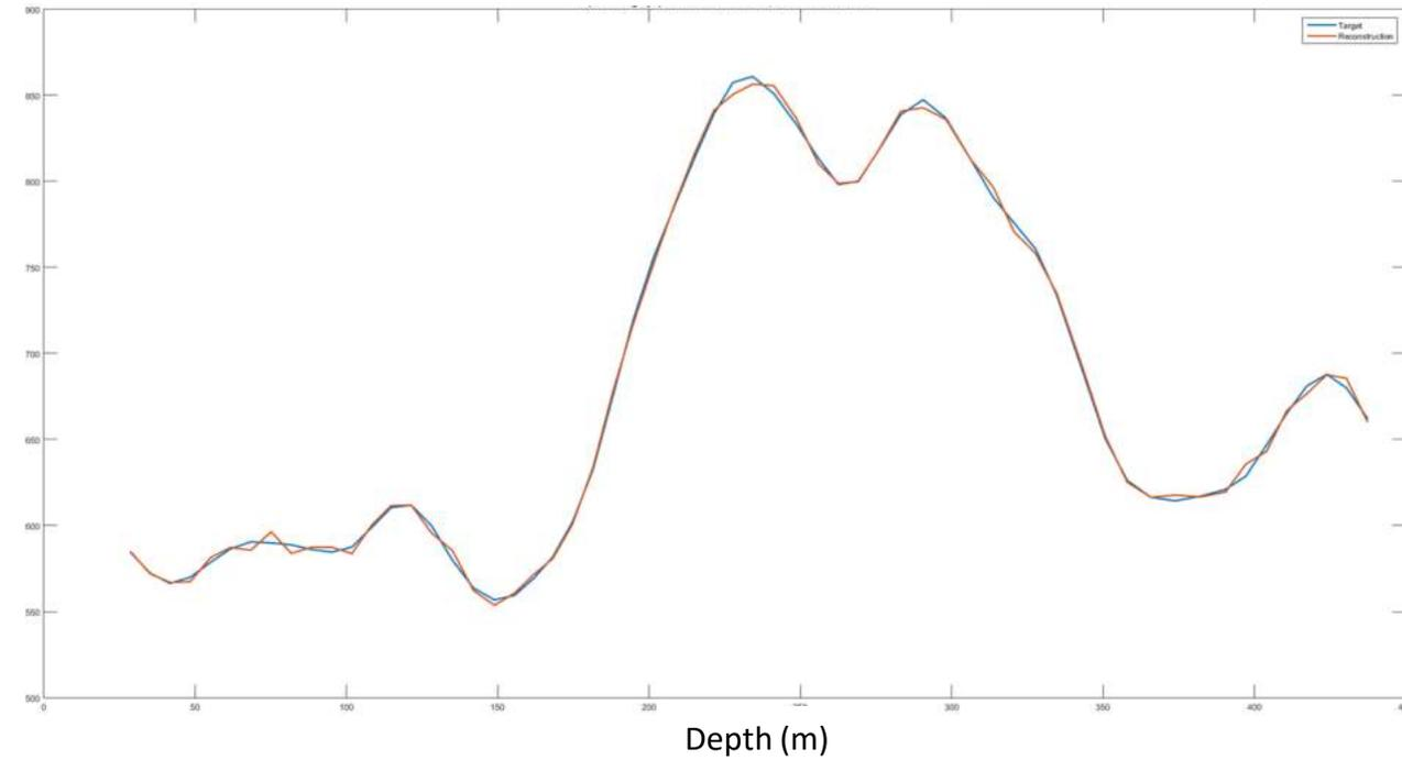
🌈 The CalcData Mix for Neutron Porosity at Bletchingley 1 shows a correlation of 98% using a 4 Smooth & correlation of 99% for an 8 Smooth.
