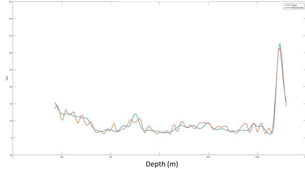
🌈 The CalcData Mix for Resistivity Short at Bletchingley 2 shows a correlation of 80% using a 4 Smooth & correlation of 97% for an 8 Smooth.
