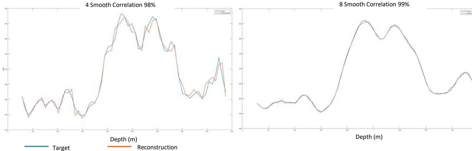
ADR data (in orange) are imported alongside training data (in blue) outputting a matching graph as well as a coefficient that used for the Calc Data Mix tool. A correlation value is also included.
